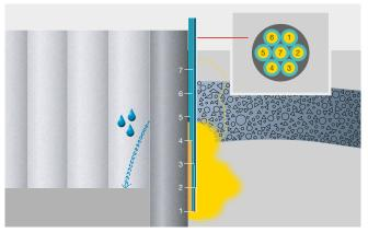
Stabilization and sealing of a bored pile wall with a graded injection tube bundle
