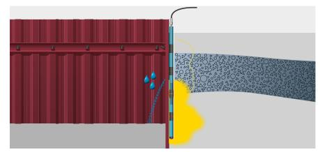
Stabilization and sealing of a sheet pile wall using the sleeve tube method
