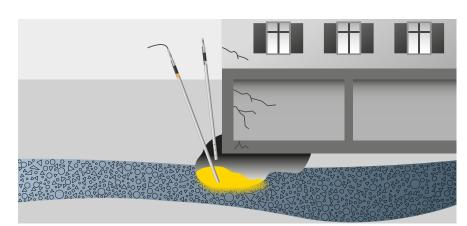
Cavity filling accessible from the outside (with injection lance)
