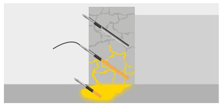
Cavity filling and consolidation in quarry stone masonry
