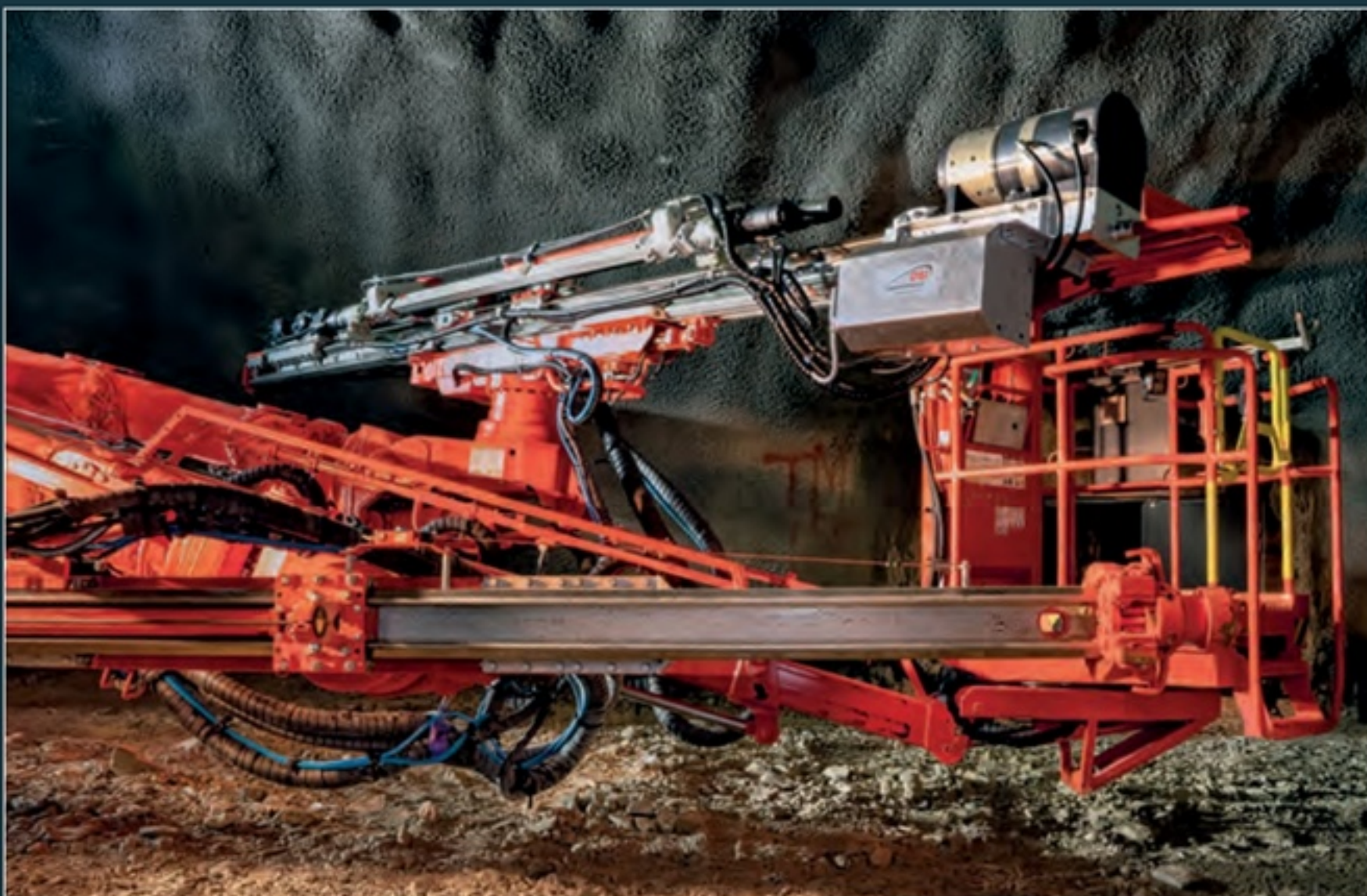
DSI's AT Pipe Umbrella System has evolved over its 25 years. On the right is an early iteration at work in the Hirschhaggen Tunnel, Germany in 2015. On the left, the latest version combining umbrella system and jumbo is seen in action at Sandvik's mine test facility in Tampere, Finland.
