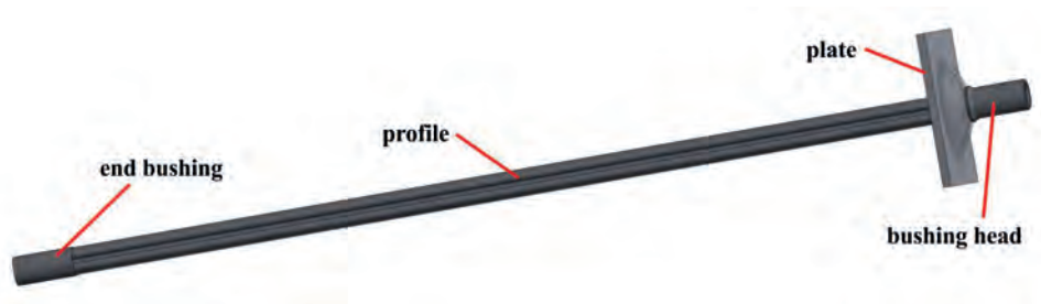
Figure 7. Typical system components of a water expandable friction bolt.
