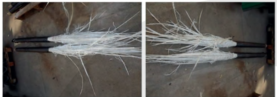
Figure 17: GFRP Bolt – exemplary sample failure after tensile test.
